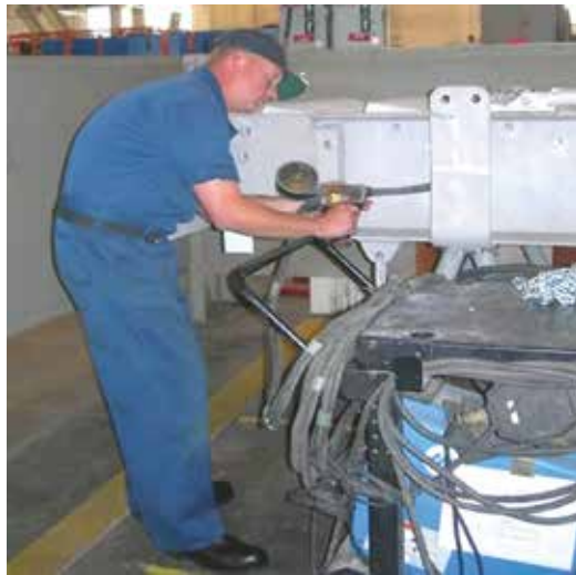
Figure 6. Welder demonstrates awkward postures which were quite common during welding tasks on the ACCOM ladder.
