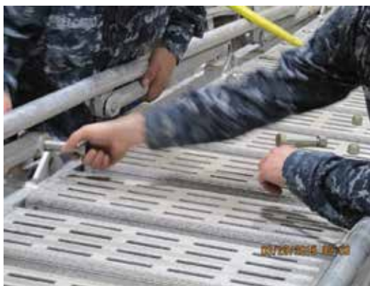
Figure 2. Assembling accommodation ladder requires long duration of highly repetitive motions while exerting force. Pneumatic tools are not allowed and therefore the exposure is combined with high and somewhat awkward hand forces.
