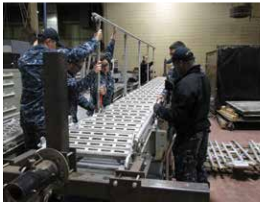
Figure 3. Assembling rails on an accommodation ladder.
