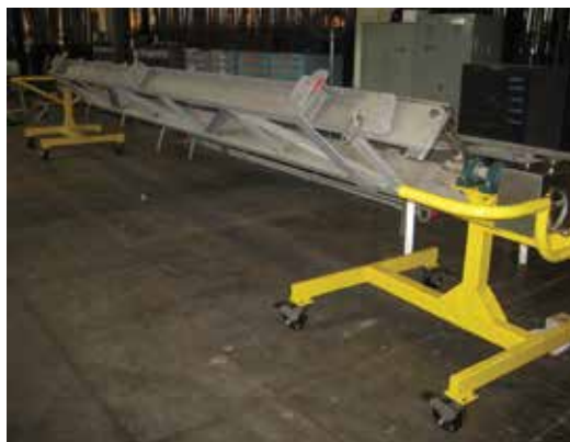
Figure 7. After the intervention, rotating ladder fixture allows one worker to safely turn the ladder and locks into place. The ladder system saves time and effort and reduces the risk of injury and equipment damage.
