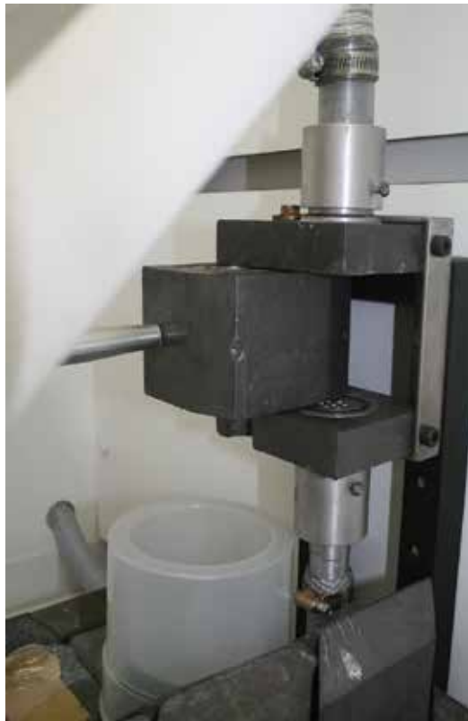
Figure 11. Shielded port for sample transfer.
