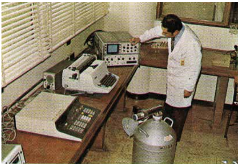
Figure 2. Neutron activation analysis instrumentation, Ge-li detection system (1971).
