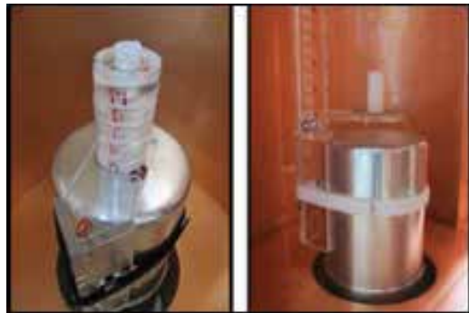
Figure 25. Detection geometry for check source verification.
