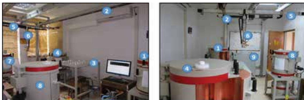
Figure 21. Positioning system: 1. Detector A; 2. X-axis linear actuator; 3. Sample rack (64 positions); 4. Detector B; 5. Y-axis linear actuator; 6. Z-axis linear actuator; 7. Detector C; 8. Detector D; 9. Control panel.
