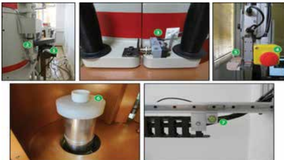
Figure 23. Positioning system: 1. Electric motor to open/close shielding; 2. Shield sensor for opening; 3. Shield sensor for closing; 4. Emergency stop; 5. Sample gripper; 6. Detector sample support; 7. Actuator motion limit sensor.
