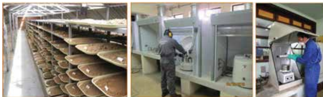
Figure 16. Sample preparation process: (a) drying (b) grinding and (c) screening.
