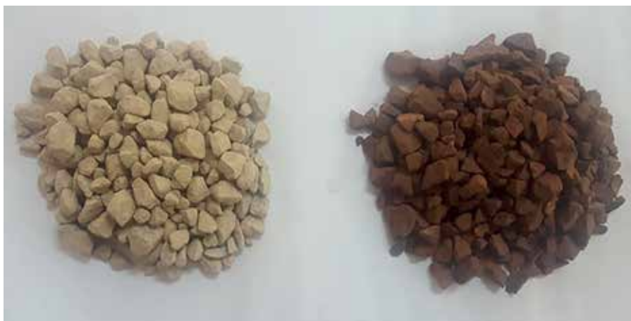
Figure 6. Raw siderite (on the left) and calcined siderite (on the right).
