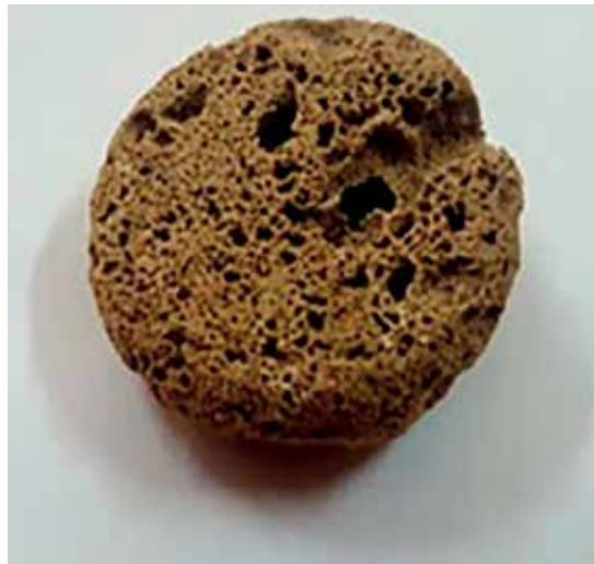
Figure 20. 30% by weight urea-added pellet obtained by microwave irradiation.
