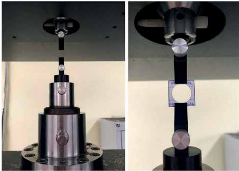
Figure 6. Single fiber disposition in the dynamometer MTS.
