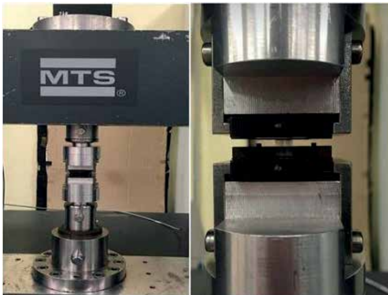
Figure 7. Pressley clamps in the dynamometer device.
