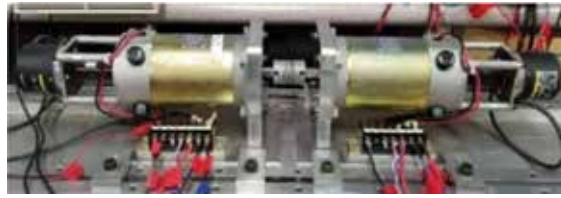
Figure 4. Photograph of the experimental two-mass resonance model.
