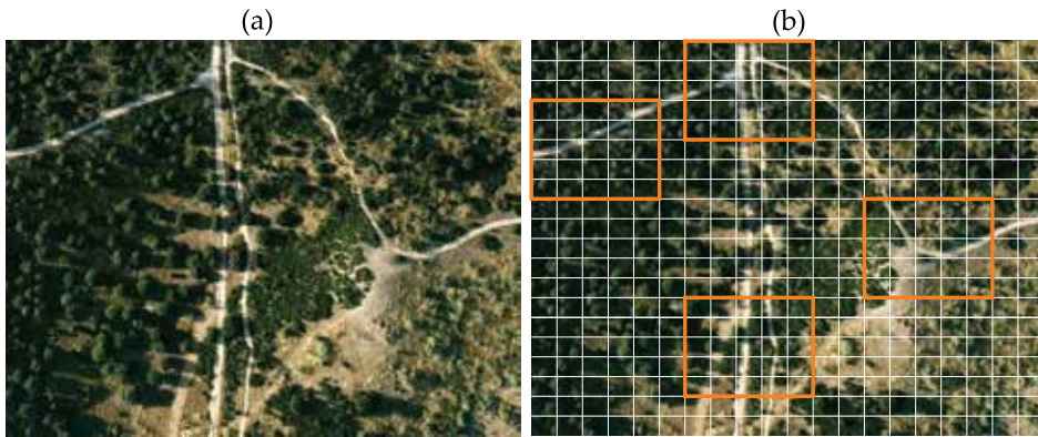
Figure 8. (a) Example of a real environment modelled as a grid map. (b) Patches of terrain used for training are marked with an orange box.
