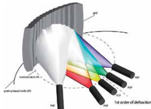
Figure 11. Rowland setup of demultiplexer.
