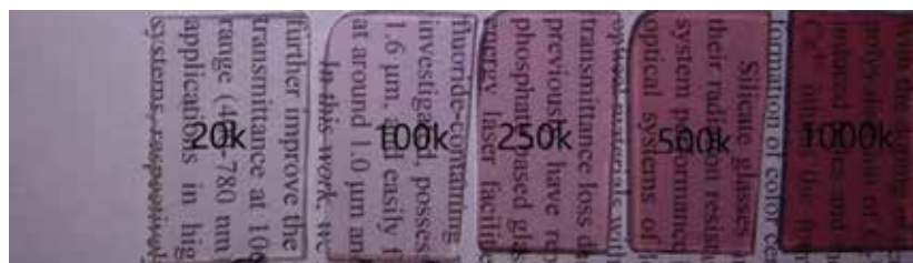
Figure 1. Photographs of a series of phosphate-based glasses with different radiation doses (20k, 100k, 250k, 500k and 1000k rad (Si)).
