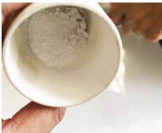
Figure 2. The BCABS-1ZrO 2 was prepared after drying in the over at 150°C for 4 h.
