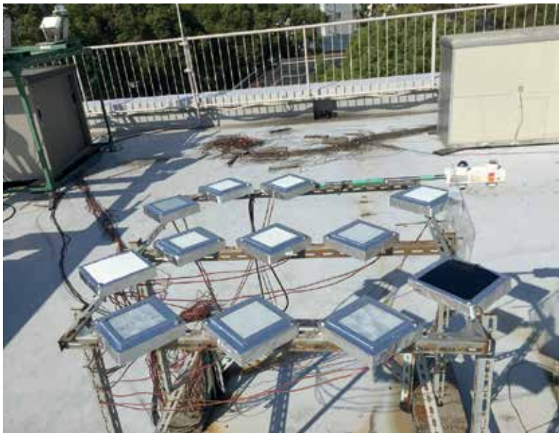
Figure 16. Experimental stand for deriving retroreflectivity of developed glass bead RR samples.
