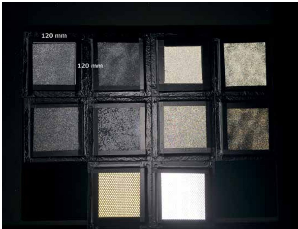
Figure 10. Retroreflection effect of developed glass bead RR materials when the artificial light source is incident on their surface.
