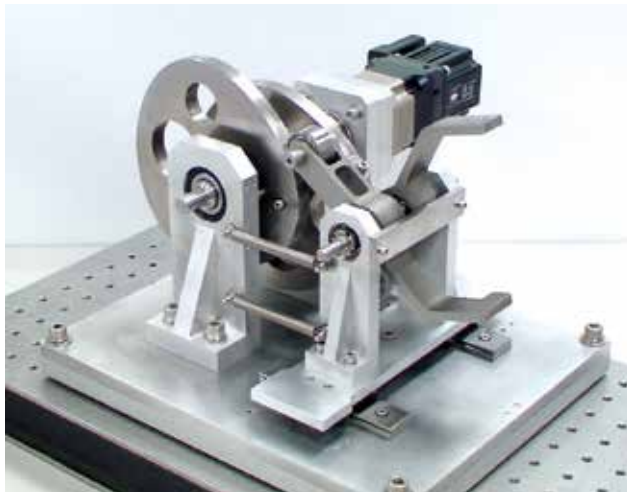
Fig. 6. Built assembled conjugate cams with measuring fixture
