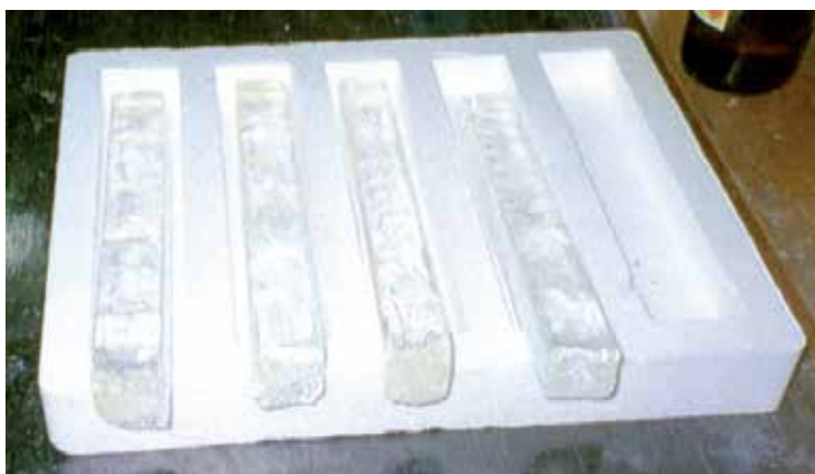
Fig. 3. Bridgman crystals. The ingot shape is given by an envelope-like crucible
