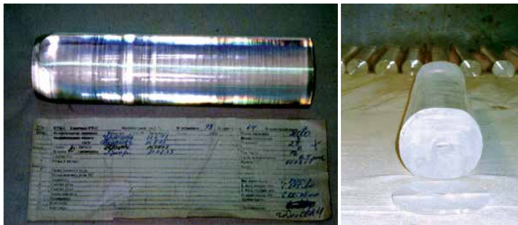
Fig. 2. Czochralsky crystals. The ingot section results from growth parameters and lattice dimensions. Important material scrap is due to difference between ingot and piece, but “peel-like” scraps are recyclable
