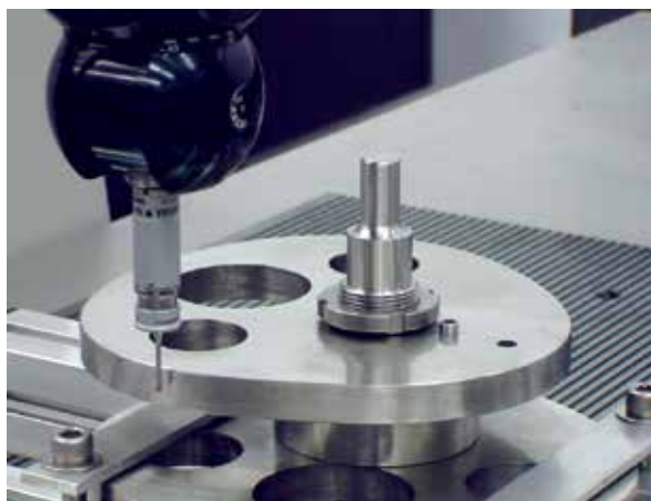
Fig. 8. Measuring the conjugate cam profiles by using a CMM
