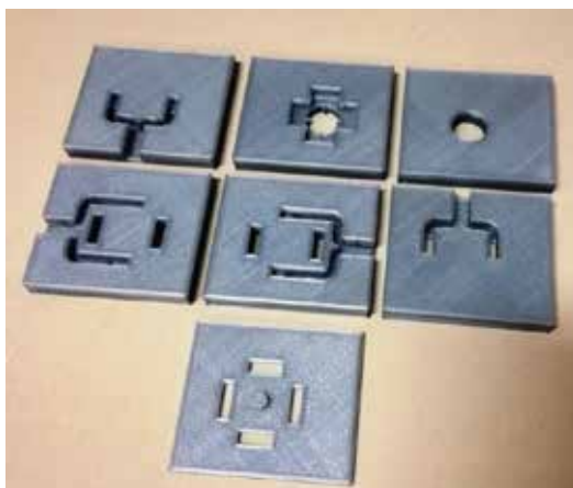
Figure 4. Printed layers of an ortho-mode transducer (OMT) based on turnstile junction, working in W-band.
