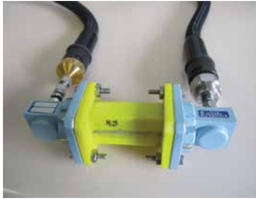
Figure 5. 3D printed WR75 waveguide section ready to be measured.
