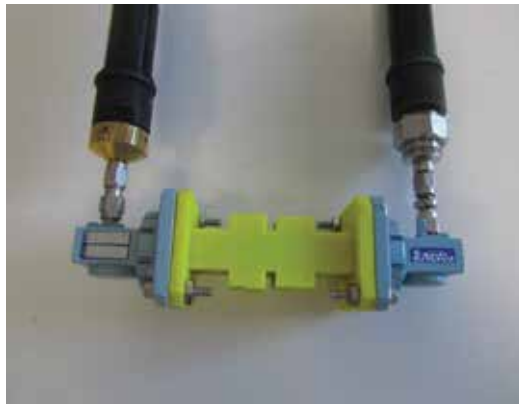
Figure 15. Measurement setup for the low-pass filter connected to the VNA.
