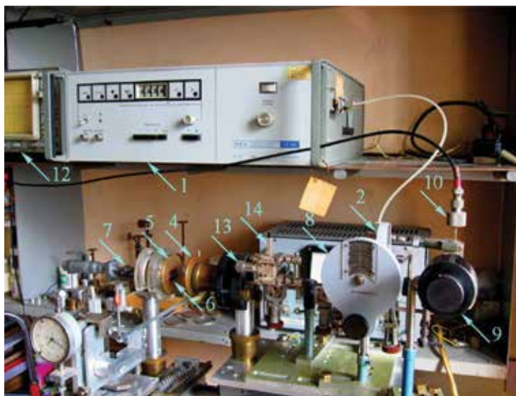
Figure 12. The photo of the OR with the segment of rectangular waveguide and the experimental unit.
