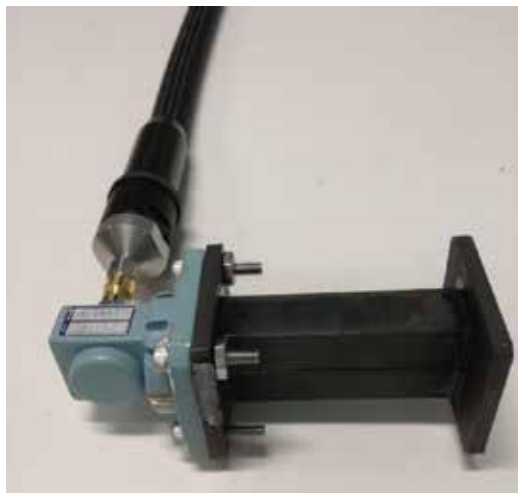
Figure 11. Measurement setup of the waveguide load.
