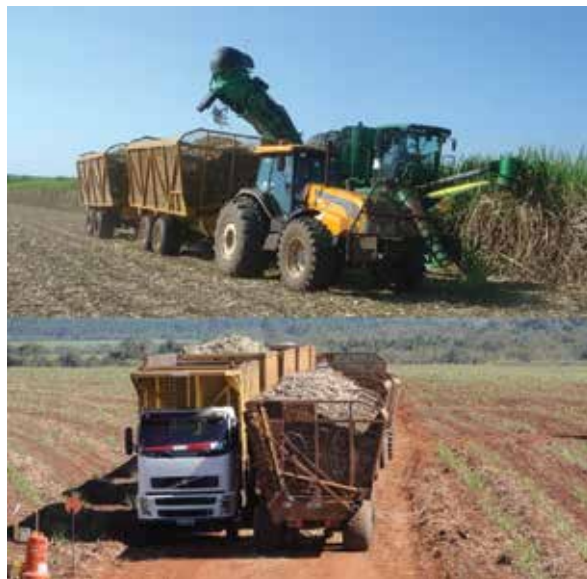
Figure 5. Transshipment to aid the transport of sugarcane from the plot to the truck or train. Credit: Luiz Carlos Dalben.
