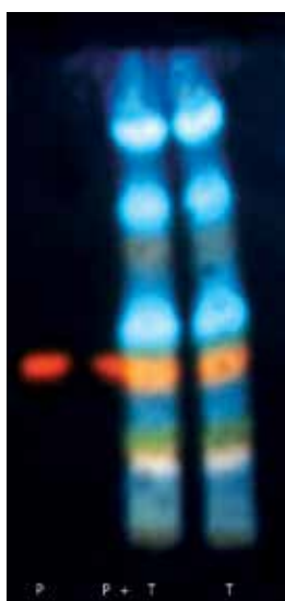
Fig. 6. TLC analysis of the tincture of Calendula officinalis L. Eluent I: ethyl acetate; formic acid; acetic acid; water (100:11:11:26); developer: NP/PEG 4000. Observation under light UV 365 nm; P- rutin standard ; T- Calendula tincture (Nunes, 2008; Nunes et al., 2009)
