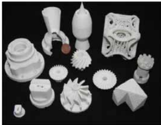
Figure 7. Pure alumina parts processed by SLM. Reprinted from [28], with permission of Cambridge University Press.
