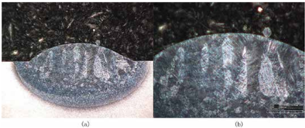
Figure 12. Ti-6Al-4V single-layer deposition grain morphology at (a) 50x and (b) 200x.
