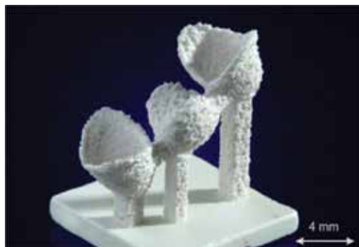
Figure 15. Direct SLM produced full ceramic framework for a dental restoration Reprinted from [54], with permission of Elsevier.
