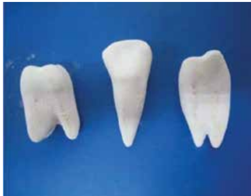
Figure 13. Teeth made by SLS under the optimized technical parameters Reprinted from [59], with permission of Emerald Publishing Limited.
