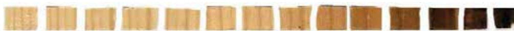
Figure 2. Color change of wood and its estimated thermal degradation (after removing charred layers, cuts of 1 mm in thickness have been made).
