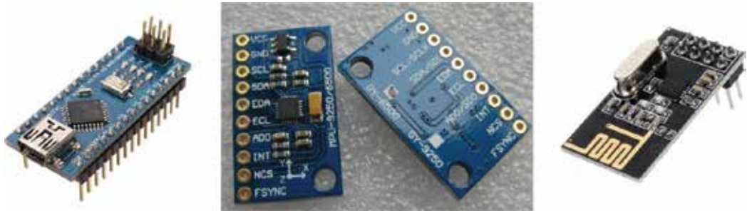
Figure 10. Arduino Nano, MPU-6500, and NRF24L01.
