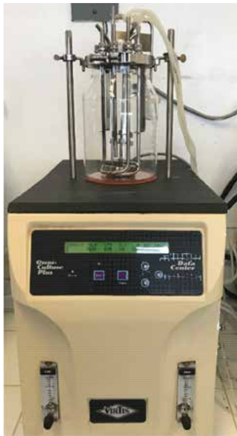
Figure 2. Chemostat Omni Culture Plus (Virtis) used for fermentation experimental process.
