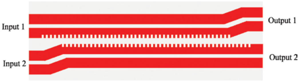
Figure 12. Schematic of a polarization-independent directional coupler based on slot waveguides with SWG structures.
