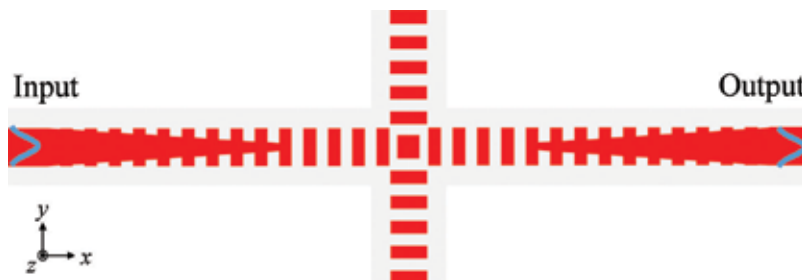
Figure 8. Top view of a SWG-based waveguide crossing.
