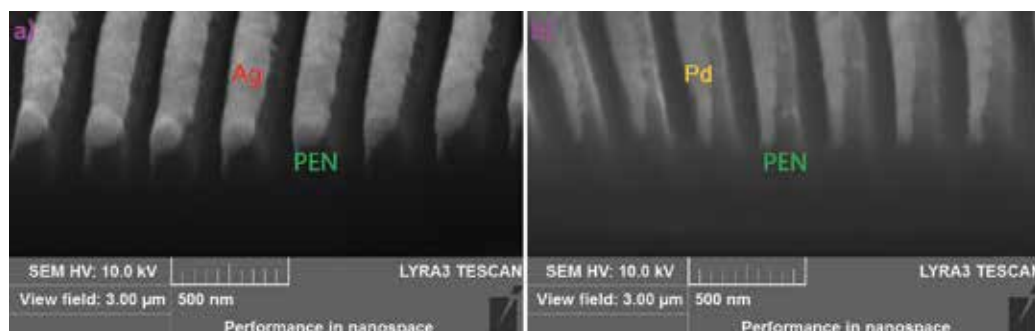
Figure 4. FIB-SEM images of (a) silver and (b) palladium NW arrays supported on laser-patterned PEN.
