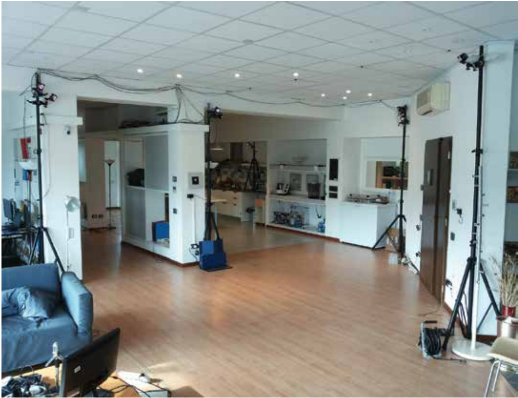
Figure 6. Part of the motion capture cameras used to cover the RoCKIn@Home area at the RoCKIn Camp held in Peccioli (Italy) in 2015.
