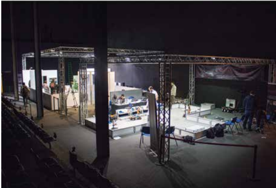
Figure 3. RoCKIn@Work test bed, including the trusses for the MCS cameras on the right.
