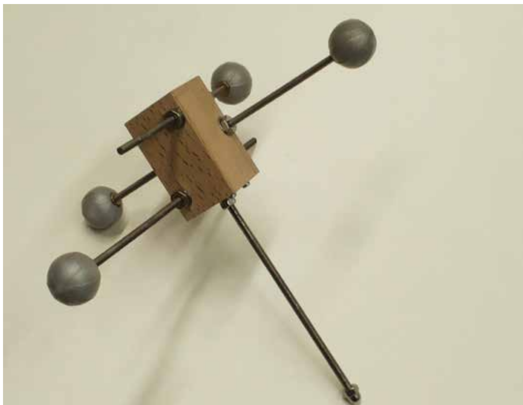
Figure 3. Marker set used for functionality benchmark ‘Control’ of RoCKIn@Work at the 2015 RoCKIn Competition.
