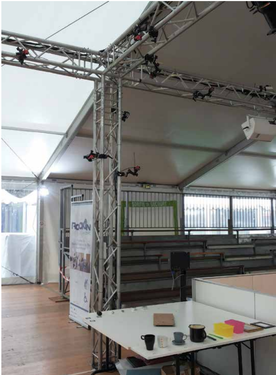
Figure 9. Setup for functional benchmark 1 (Object Perception) at the 2014 RoCKIn Competition in Toulouse, France. The (red) motion capture cameras used to track the objects presented to the robot are mounted on the metal truss adjacent to the table.
