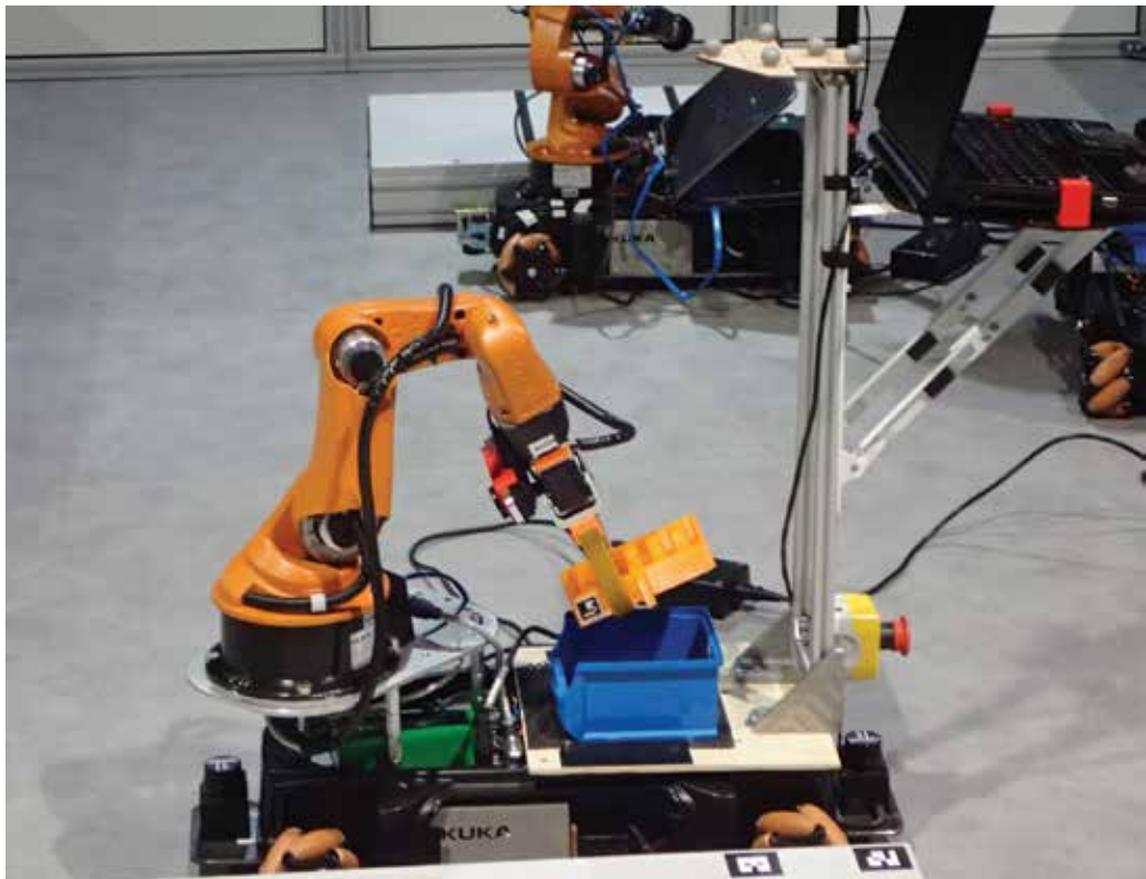
Figure 6. Placing an assembly aid tray into small load container.
