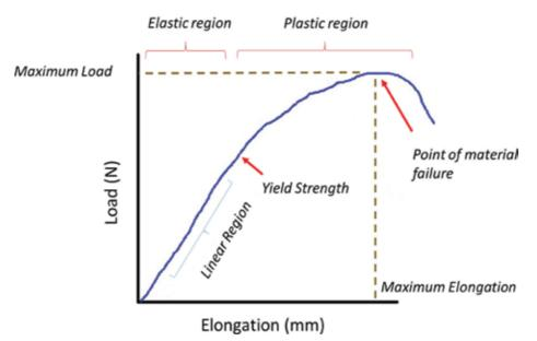
**Figure 2.** Defining the basic mechanical properties of a material by uniaxial mechanical testing. The 'maximum load' is the maximum amount of stress that a material can bear before it fails. The 'maximum elongation' is the maximum strain a material can achieve before it fails. The 'yield strength' is where irreversible deformation to the material starts.
