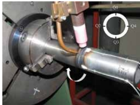
Figure 3. TIG welding of the tubular specimens with temperature measurements [8].
