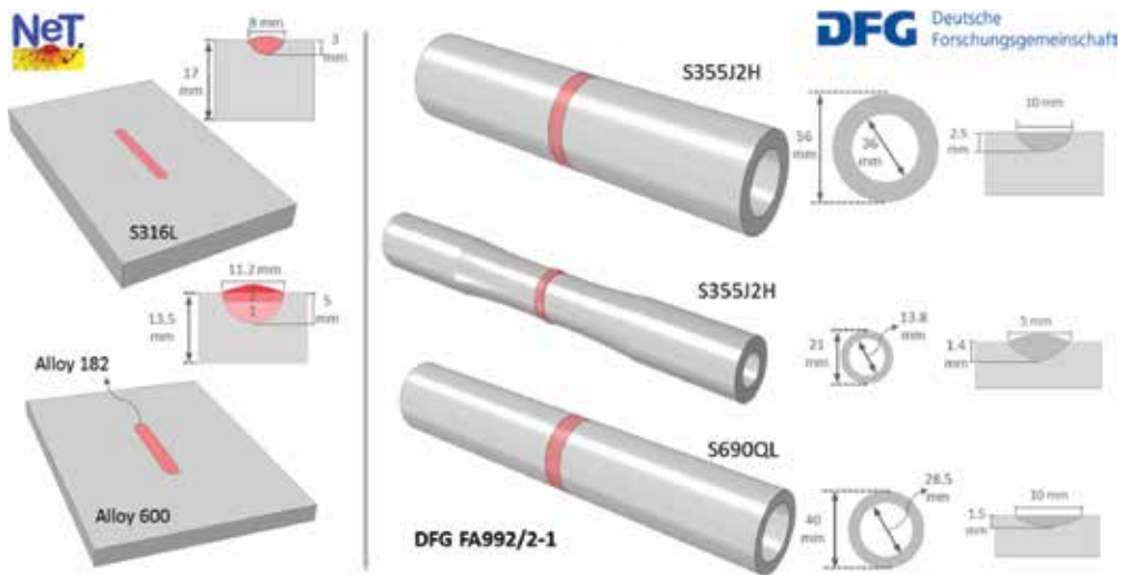
Figure 2. Simulation studies and residual stress measurements: cooperation in NeT (left), investigations within the project by German Research Foundation (DFG) (right).
