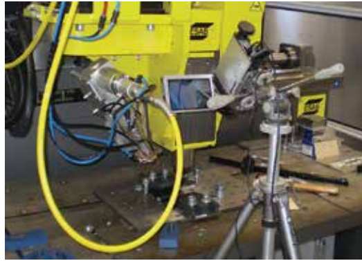
Figure 4. Thermographic experimental setup.
