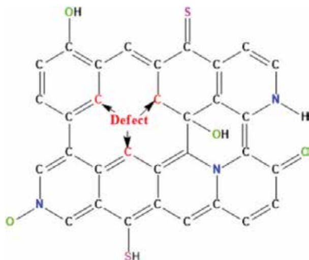
Scheme 2. Aromatic carbon lattices can embrace many types of heteroatom doping such as nitrogen (blue), oxygen (green), sulfur (pink), and so on. Defective carbon sites (red) that are unsaturated can also be treated as anchoring sites for ions.
