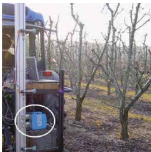
Figure 14. LIDAR placed on the back of a tractor [28].
