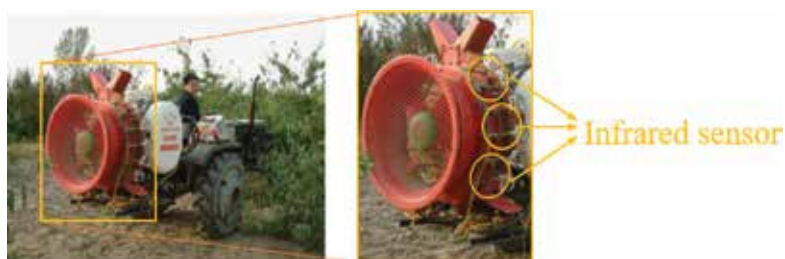
Figure 1. Photo of the automatic target-detecting orchard sprayer working in orchard [6].
