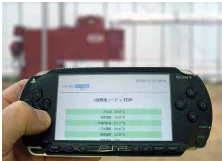
Figure 4. Managing the node for an oil air heater using a portable game console in a greenhouse using an UECS.
