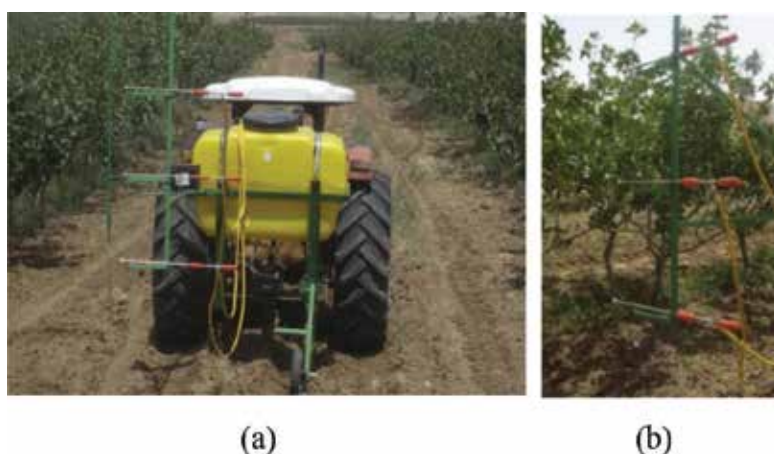
Figure 10. (a) Variable-rate sprayer for fruit tree protection, (b) attached nozzles mounted on the vertical masts for orchard tree spraying [29].
