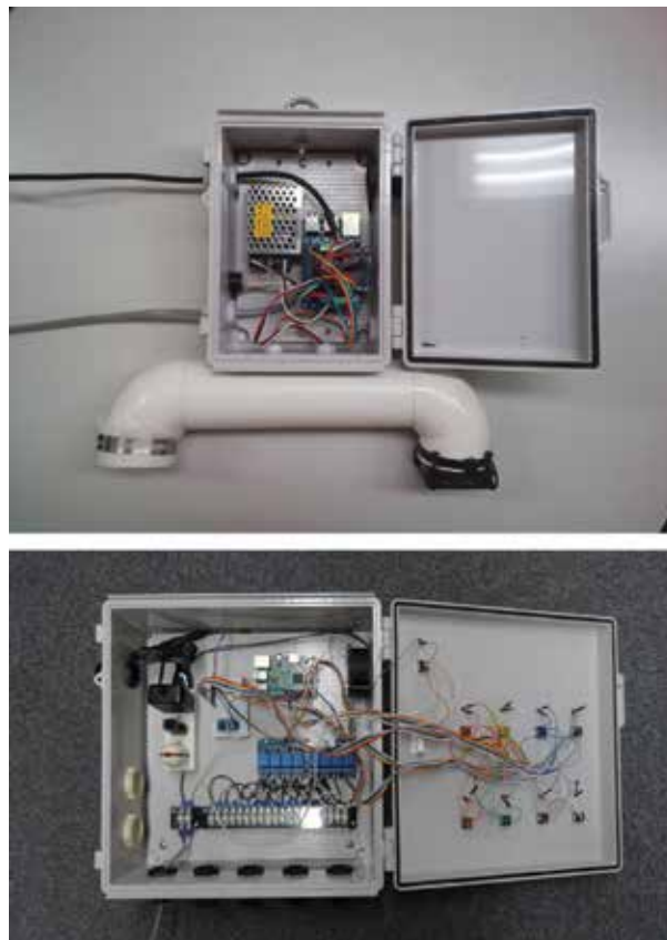
Figure 9. The UECS DIY node completed by the workshop. Upper: sensor node for measuring greenhouse climate, lower: relay node for controlling actuators such as open-close motor of roof ventilators.
