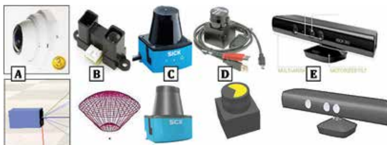
Figure 8. Major sensors used in the experiments, first row image are the actual and the second row images are the simulated sensors.
