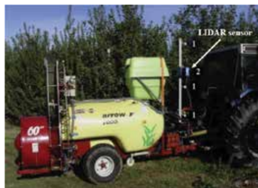
Figure 13. Variable-rate orchard sprayer prototype implemented with LIDAR sensor [13].
