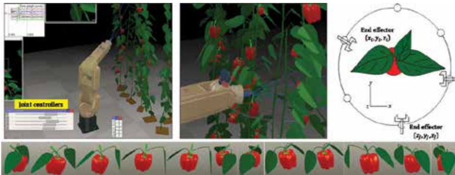
Figure 20. Two dimensional scanning experiment ( x - y , x - z , and y - z planes) for finding the maximum fruit visibility. Camera was set to move at 30 degrees increments around the fruit and plant model.
