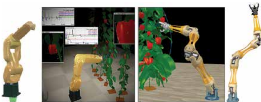
Figure 11. Simulation scene setup with CAD models of the professional robot manipulator used in visual servo control experiment, left: Fanuc LR Mate 200iD, right: NOVABOT.
