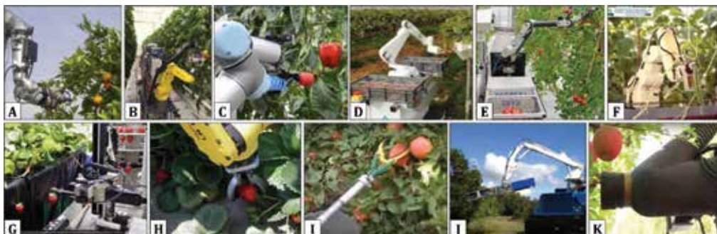
Figure 2. Research and development in robotic harvesting of fruits with different manipulators and gripper mechanisms for: (A) citrus, (B, C) sweet pepper, (D, E) tomato, (F) cucumber, (G, H) strawberry, and (I–K) apple.
