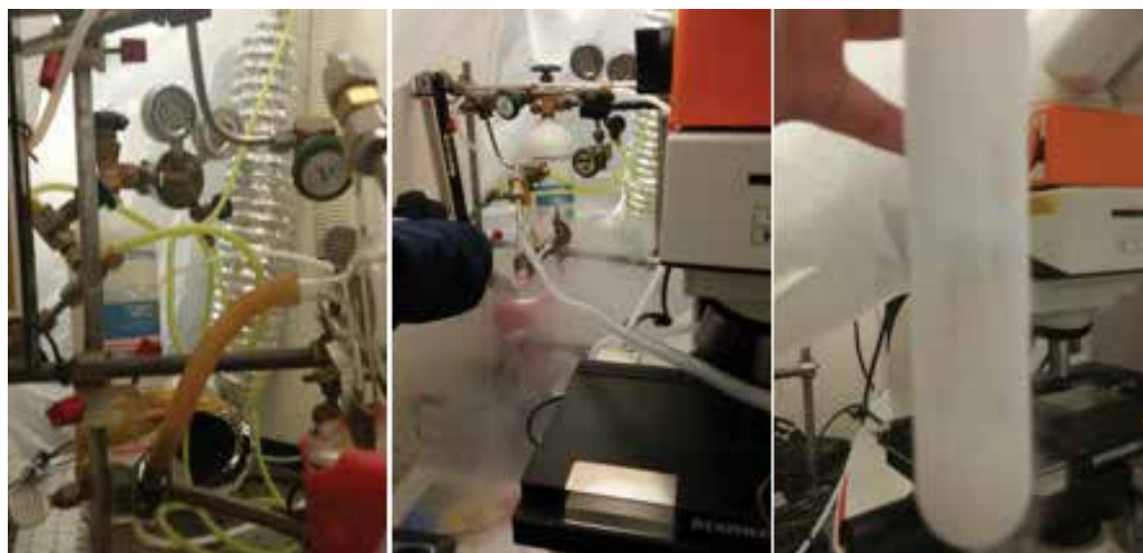
Figure 4. Left: Setup showing the tubing layout for the gas exposure Raman spectroscopy experiments; center: Filling the bubbler with liquid nitrogen to break up dangerous gas components; right: Bubbler after experiments had concluded [7].
