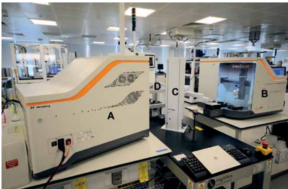
Figure 8. Automation platform used with our iQue® Screener HD. (A) and (B) iQue® Screener HD, (C) ACell robotic arm, (D) NanoServe™ stacker carousel.
