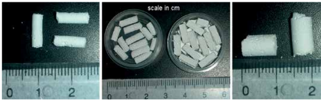
Figure 7. Hydroxyapatite objects molded in different sizes and shapes by the modified gelcasting process (scale in cm).
