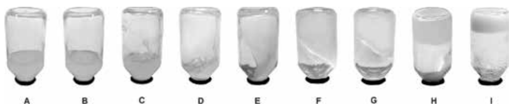
Figure 3. Bottle testing characterization of PAM-PEI hydrogels using the Sydansk's gel-strength code.
