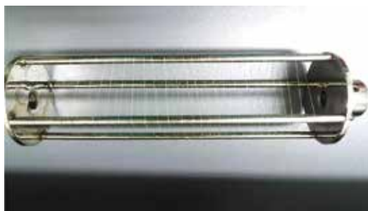
Figure 6. The capability of producing unlimited length of coaxial Chit-Alg (1) fibers as shown onto a collector. [11] Reproduced with permission. 158 Copyright 2015, Wiley-VCH.
