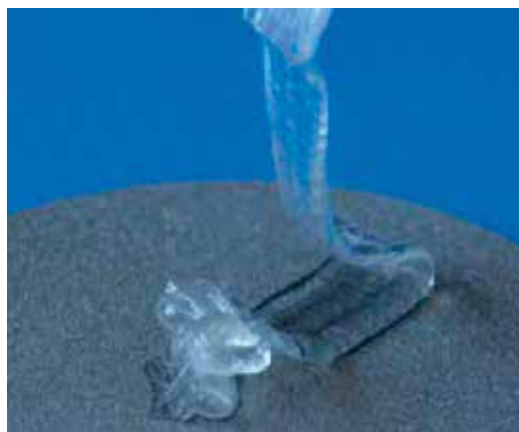
Figure 2. DAC ® HA-g-PLA, fast-resorbable, hydrogel coating. Composed of covalently linked hyaluronan and poly-D, L-lactide, the “Defensive Antibacterial Coating” (DAC ® , Novagenit Srl, Mezzolombardo, Italy) is the first antibacterial-coating cleared for clinical use in orthopedics, trauma, dentistry and maxillofacial surgery in Europe.
