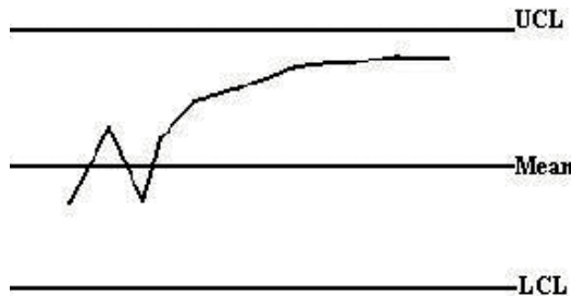
Figure 29. Example of a control chart showing an approach to UCL or LCL pattern.
