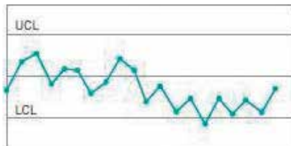
Figure 25. Example of a control chart showing a shift in process level pattern.
