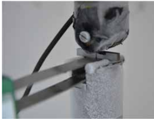
Figure 18. KLST specimens ( 4 \times 3 \times 22 \text{ mm}^3 ) from material 15CH2NMFA.
