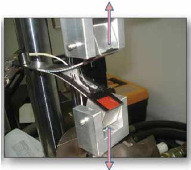
Figure 7. Illustration of the extended bridging phenomenon of the SP interleaf between the upper and the lower adjacent surfaces during mode I tests.
