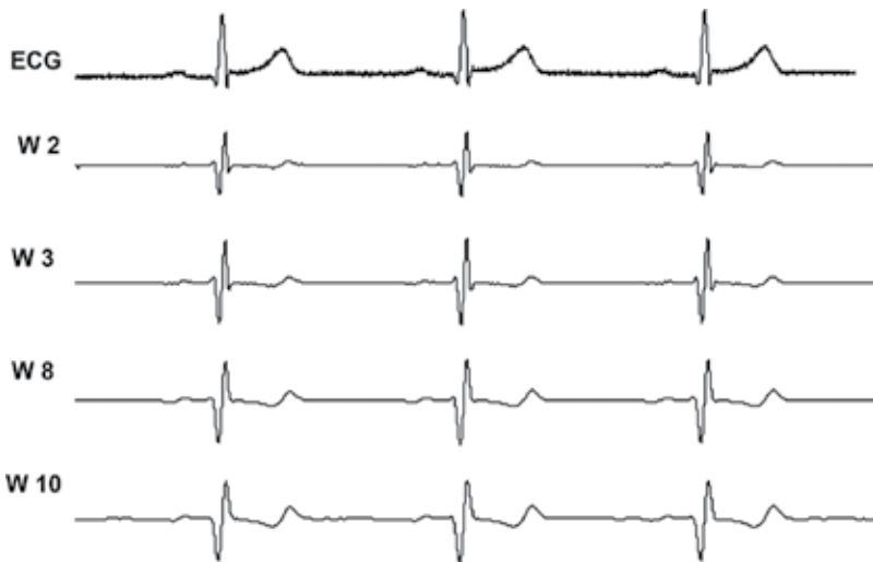
Figure 4. ECG and its CWT at scales 2, 3, 8 and 10.
