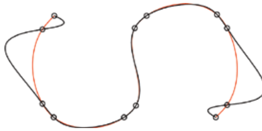
Figure 4. We interpolated with a Bèzier (black) and a cubic B-spline (red) curves.
