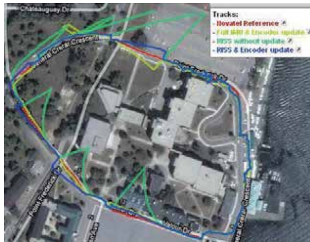
Fig. 9. Three solutions and reference for second trajectory: Red for reference, Yellow for KF using full IMU with velocity updates, Green for KF using RISS without updates, Blue for KF using RISS with velocity updates.
