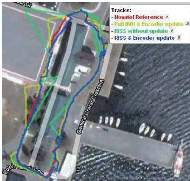
Fig. 6. Three solutions and reference for first trajectory: Red for reference, Yellow for KF using full IMU with velocity updates, Green for KF using RISS without updates, Blue for KF using RISS with velocity updates.
