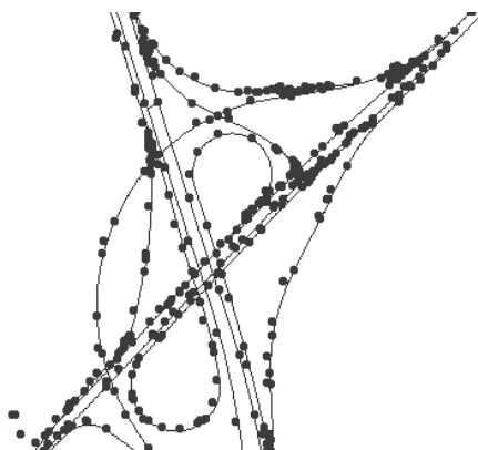
Fig. 2. GPS Data Points Collected by a Vehicle While Traveling at a Highway Interchange
