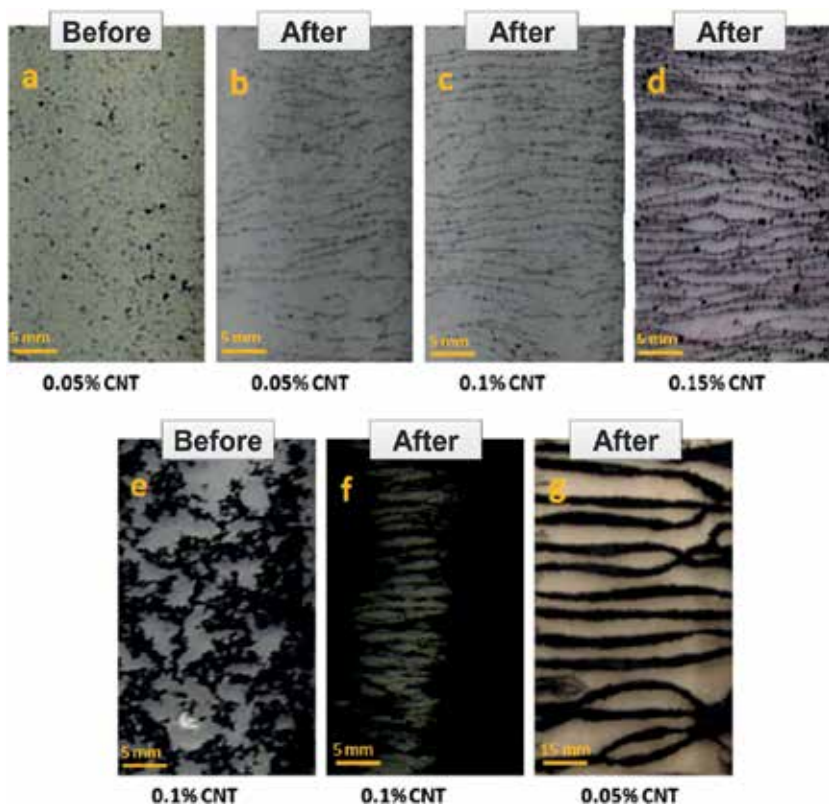
Figure 4. Optical images from aligned CNT networks with respect to their concentration, size and duration which DC electric field was applied between electrodes, (a–f) 100 V/cm for 30 min and (g) 200 V/cm for 30 min [3].
