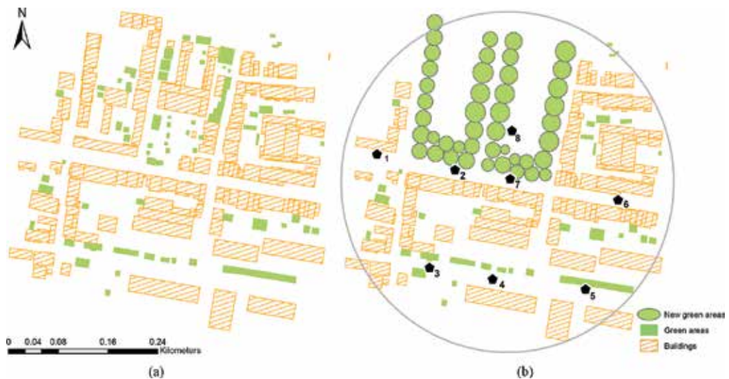
Figure 2. Computational domain for (a) the baseline scenario and (b) the green scenario, including the wind speed measurement point location, or the corresponding computational cells in the CFD simulations. The newly implemented green areas are represented by green circles.
