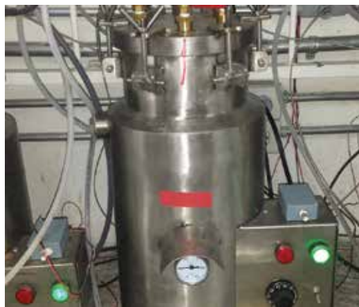
Figure 1. Laboratory-scale anaerobic reactor with pumped circulation.
