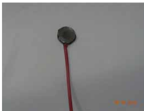
Figure 1. The photograph of the CuO-graphene electrode.
