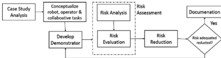
Figure 1. Overview of the demonstrator-based design methodology employed to ensure a safe collaborative workstation.
