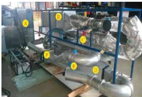
A - Chiller, B - PVT emulose, C - PCM fan, D - TES, E - Damper, F - Heat exchanger
