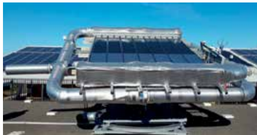
Figure 4. Illustration of the laboratory-scale PVT test rig.
