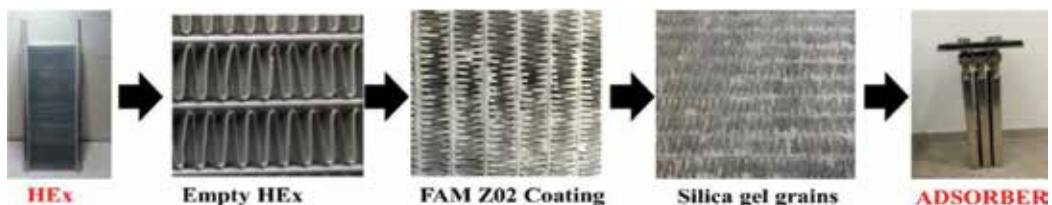
Figure 8. Adsorbers’ manufacturing procedure [55].
