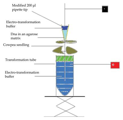
Fig. 3. Diagrammatic illustration of the electro-transformation equipment and experimental set-up
