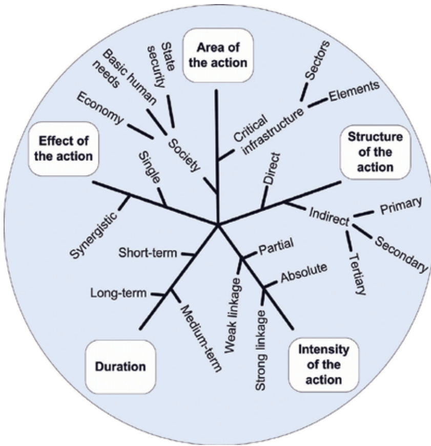
Figure 3. Aspects that create the character of impacts in a critical infrastructure system [3].
