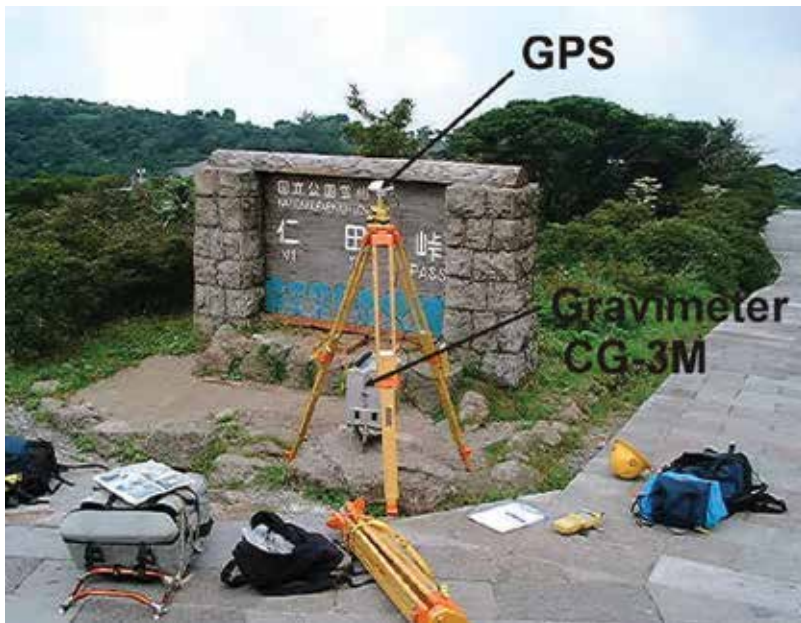
Figure 9. Photograph showing the Scintrex CG-3M gravimeter and GPS antenna at Nita station (Unzen volcano, southwestern Japan) [7].
