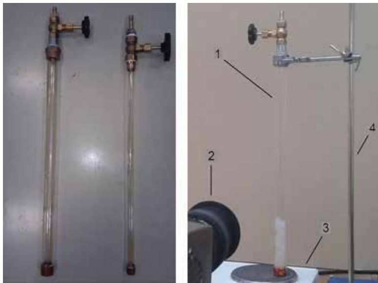
Figure 21. Working fluid flow visualisation in gravity heat pipe: (1) heat pipe, (2) video camera, (3) heat source, (4) stand.
