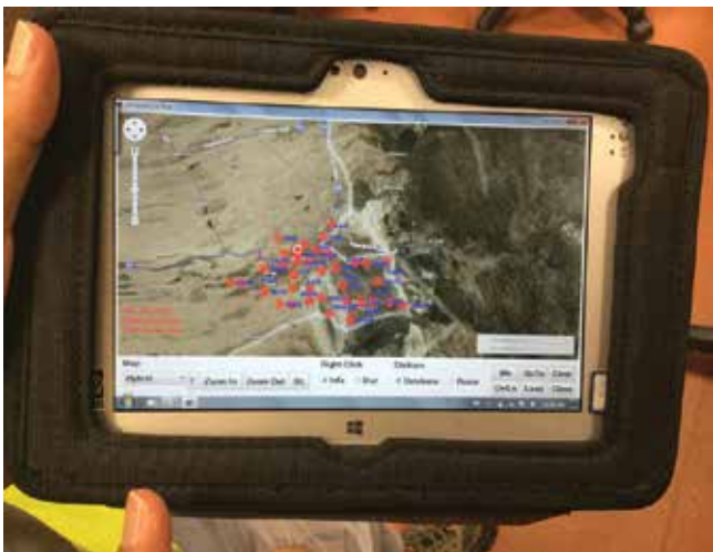
Figure 12. View of lynx LG software (Scintrex, 2017) showing the gravity stations in Alain city, United Arab Emirates, during field survey in Al-Ain city in June 2017. Lynx LG software includes data pre- and postprocessing that helps users to get a simple Bouguer gravity map of the study area just after finishing the measurements [7].
