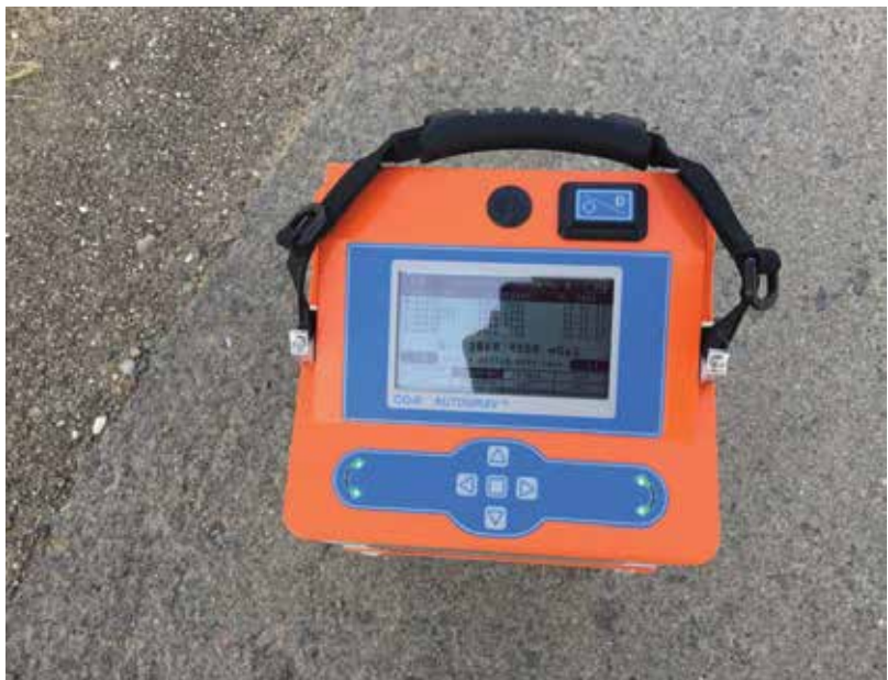
Figure 11. Top view of CG-6 gravimeter during field measurement in Alain city, United Arab Emirates (June 2017) [7].
