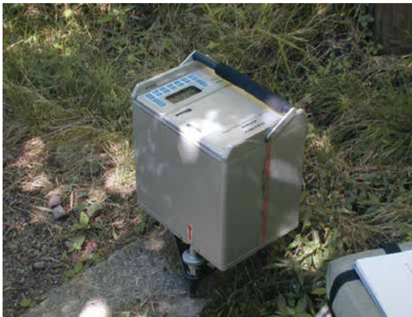
Figure 10. Photograph of CG-3M Autograv automated gravity meter. The features of this gravimeter are: resolution mGal = 0.001 ( =1 \mu Gal ), standard deviation: <5 \mu Gal , automated corrections: tide, instrument tilt, temperature, and rejection [7].
