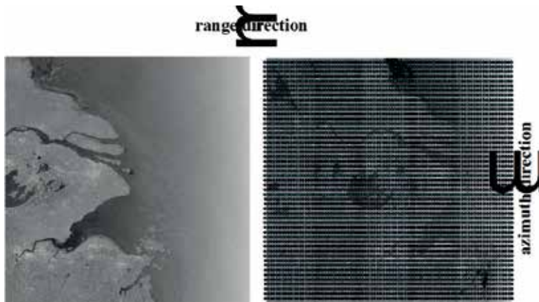
Figure 2. The NRCS of ASAR WSM scene over Yangtze estuary on 31 January 2005 (left) and 5 February 2005 (right). Superimposed points on the right plot are the Doppler centroid grids. Arrows denote azimuth and range directions of ASAR image.
