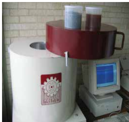
Figure 7. Low background scintillation detector NaI (TI), 325 Lab, D building, Faculty of Chemistry, UNAM.
