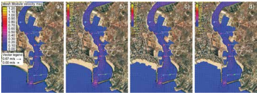
Figure 18. Modeling with the new layout. Results for the flood tide: (a) 58, (b) 59, (c) 60 and (d) 61 hours.
