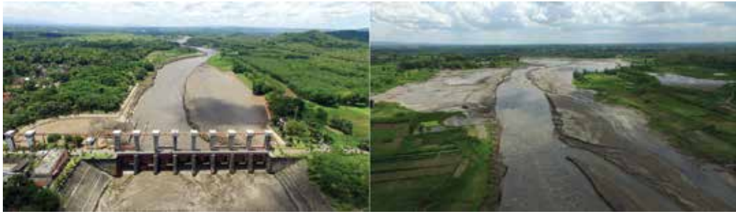
Figure 5. Aerial views of Wlingi (left) and Lodoyo (right) reservoirs taken by a drone showing sediment deposition in the reservoirs during sediment flushing on 25–26 March 2016.
