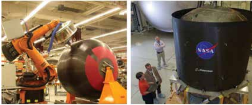
Figure 8. 2.4-m diameter tank, a robotic arm applies composite laminate [21, 22].
