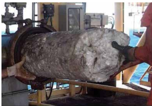
Figure 1. Recovered gas hydrate plug from a subsea pipeline off the coast of Brazil (courtesy of Petrobras).
