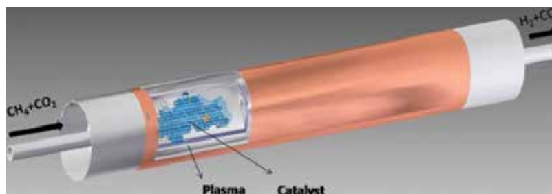
Figure 7. Schematic representation of the catalyst-packed dielectric barrier discharge reactor [29].
