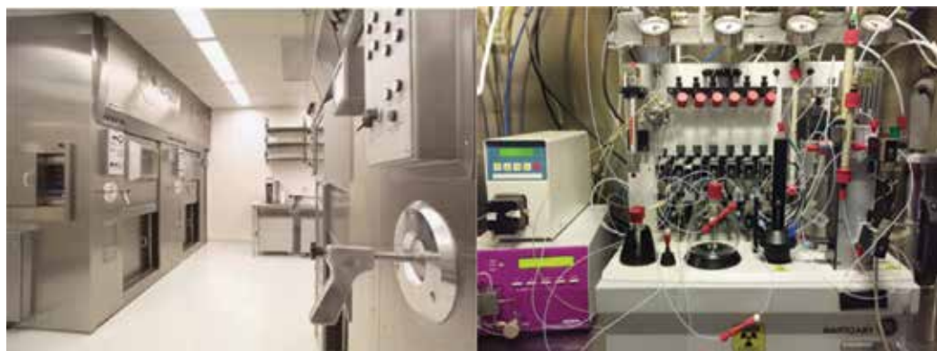
Figure 2. Automatic synthesis equipment in lead-shielded fume hoods.
