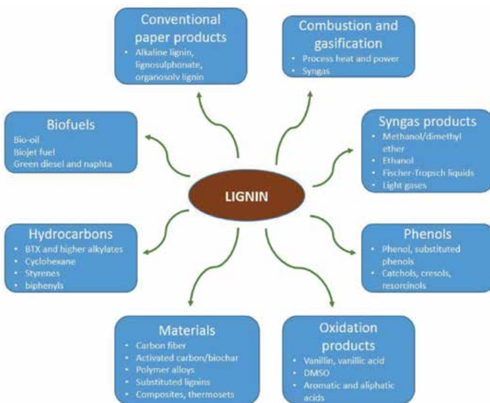
Figure 12. Scheme of conventional and potential products from lignin. BTX: benzene, toluene and xylene isomers and DMSO: dimethyl sulfoxide.
