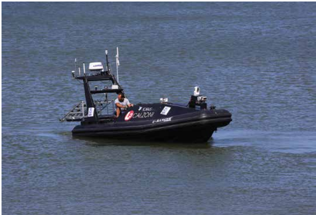
Figure 1. Calzoni U-Ranger USV (source: ICARUS).
