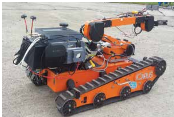
Figure 10. ICARUS COM tools installed on a small unmanned ground vehicle. (Source: ICARUS).
