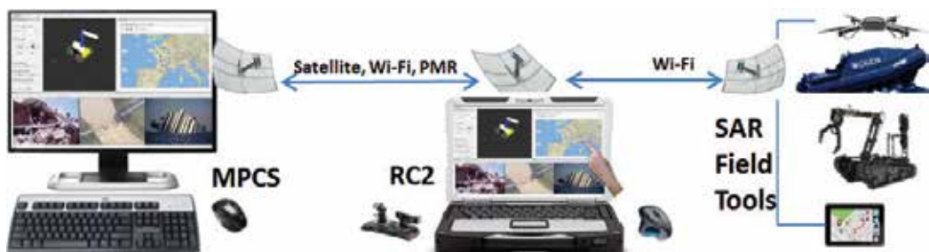
Figure 1. C2I deployment and communication framework (source: ICARUS).
