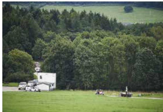
Figure 14. B-FAST team advancing with all ICARUS tools: large UGV (driving in front), small UGV (packed on first vehicle), rotorcraft (airborne in the middle of the picture) and fixed wing aircraft (airborne, but not visible in this picture) (source: ICARUS).
