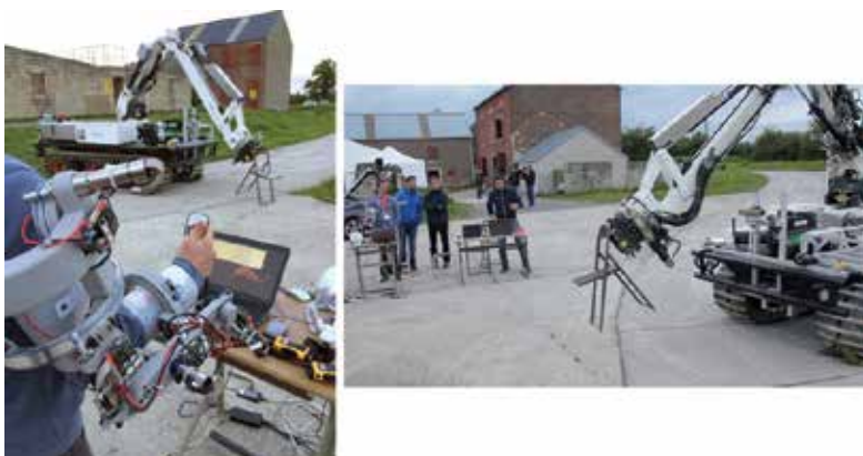
Figure 50. Control of the LUGV with the exoskeleton interface to grab objects (source: ICARUS).
