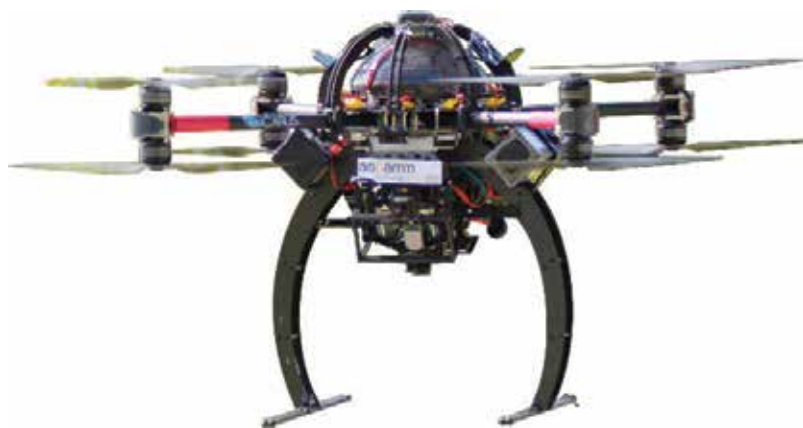
Figure 7. The Eurecat coaxial-quadrotor with the camera payload (source: ICARUS consortium).
