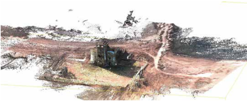
Figure 16. 3D map of the crisis area, obtained by combining 3D maps from the aerial and ground platforms (source: ICARUS).
