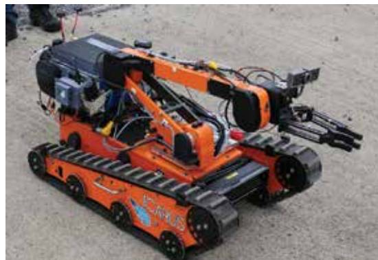
Figure 3. Small unmanned ground vehicle (Source: ICARUS).
