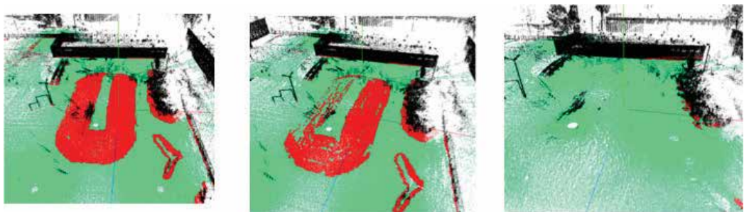
Figure 37. The traversability analysis: traversability for UGV with 10° max slope, 18° max slope and 44° max slope (source: ICARUS).
