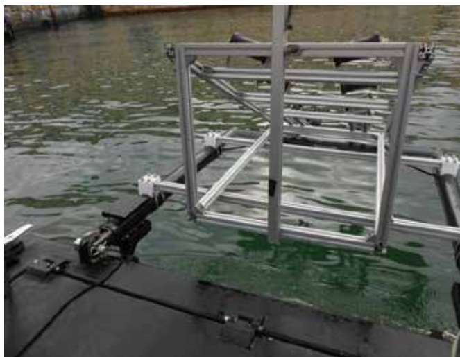
Figure 12. Deployment system installed on the U-RANGER USV (source: ICARUS).
