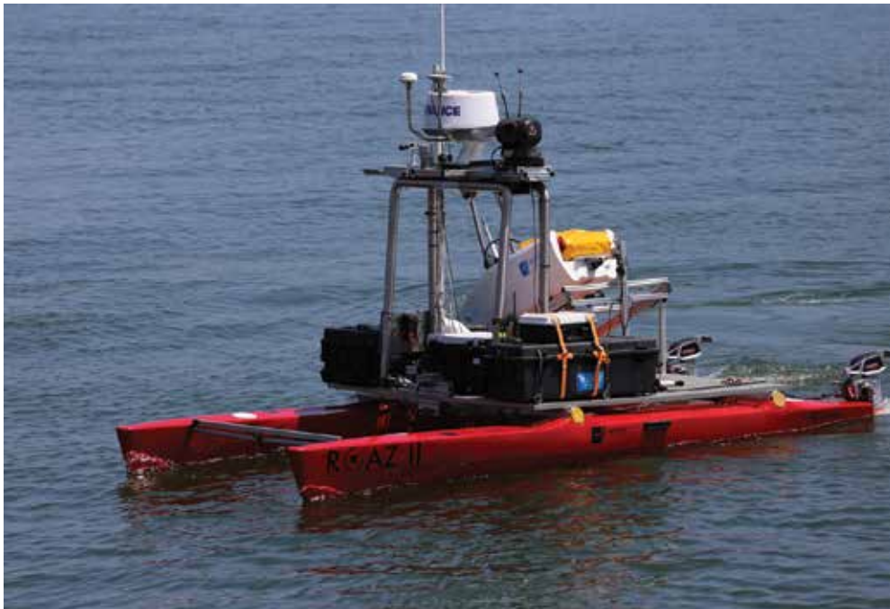
Figure 4. Roaz II USV (source: ICARUS).
