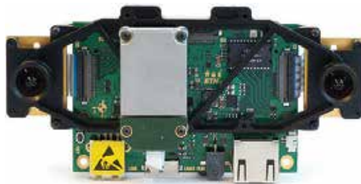
Figure 2. VI sensor hardware with two visual cameras and mounted IMU (source: ICARUS consortium).
