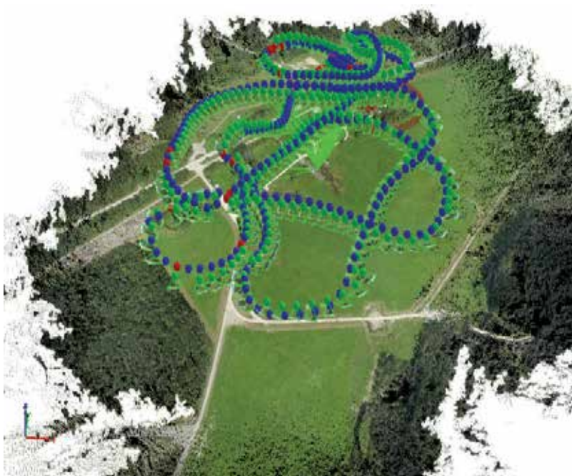
Figure 5. Optimal path planning for the AtlantikSolar UAS. The path is optimal to cover the trial site in Marche-en-Famenne. The images are used to form the shown map (source: ICARUS consortium).
