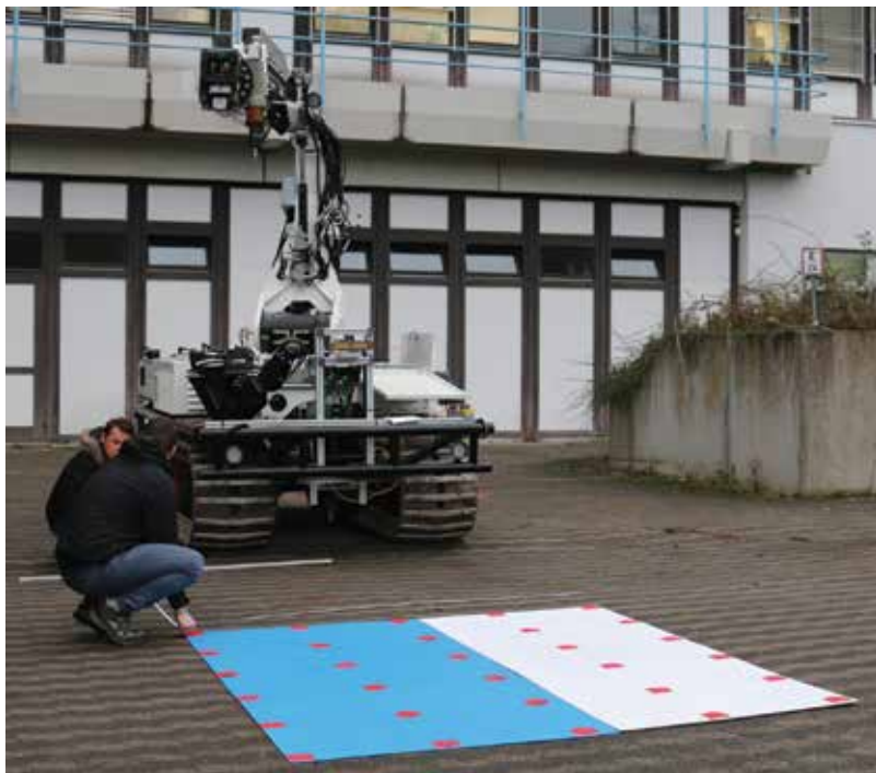
Figure 12. Calibration of the 3D vision sensor. The sensor can be seen mounted on the sensor tower of the LUGV (Source: ICARUS).
