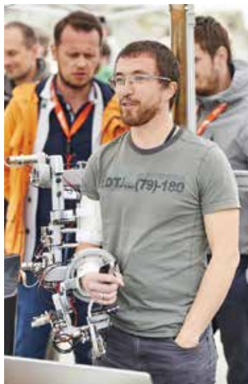
Figure 25. Remote operator using an exoskeleton to operate the manipulator arm of the small UGV (source: ICARUS).
