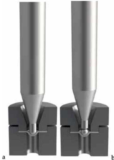
Figure 5. Schematic diagrams of the punch geometries for (a) one piece punch and (b) ball-punch configuration.
