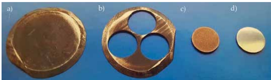
Figure 3. (a) Scoop sample, (b) scoop sample after EDM, (c) SP samples obtained through EDM and (d) polished SP specimen ready for testing.
