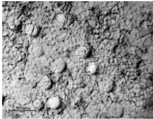
Figure 10. TEM of Waspaloy microstructure after tensile testing [50].
