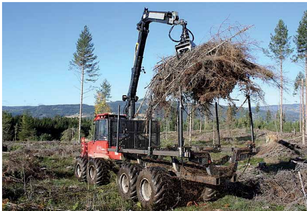
Fig. 2. Removal of a pile of branches and tops six months after harvesting, Gaupen, Norway (photo: Kjersti Holt Hanssen, Norwegian Forest and Landscape Institute)
