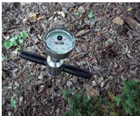
Fig. 7. Measurement of soil resistance by penetrometer
