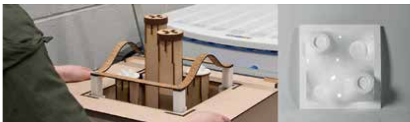
Figure 6. REM for thermoforming plastic panel [images by Frances White, Alex Morse & Maryam Bennani].
