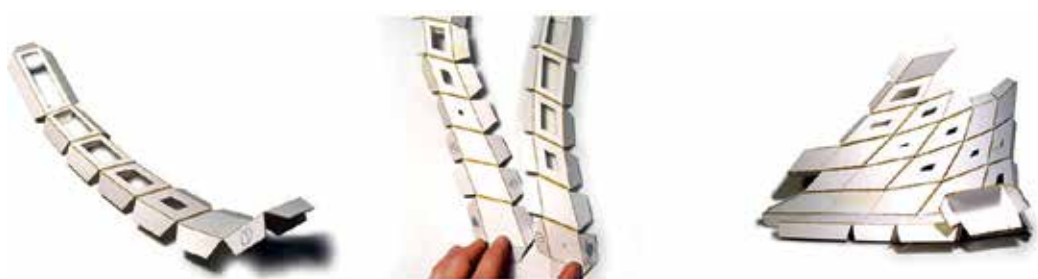
Figure 5. Laser-cut panels made with dexterity and craftsmanship using digital technology [images by Singleton, Tibballs and Yoannidis].
