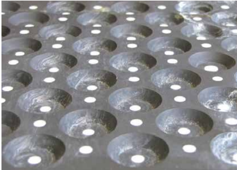
Fig. 4. Multi-level target of 270 x 190 mm with white dots and black background.
